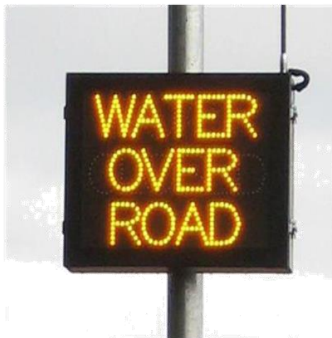
Figure 4 - Automated LED variable message warning signs
