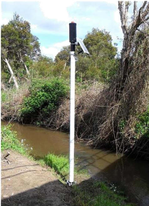
Figure 1 –Automated River Height Monitoring Station (Basic Option)
